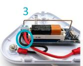
4. Insert the **black wires** to the **first terminal block (GND)** and the **red wires** to the **second** .
