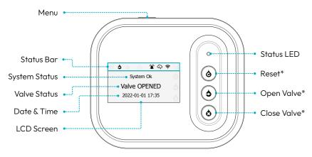
\*Only lit up buttons are active. Depending on system state, buttons behavior might change. The new behavior will be identified on the LCD screen beside the buttons.
