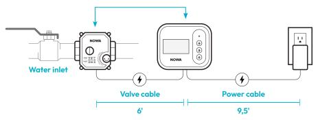
The NOWA valve cable length is 6 feet and the control panel power cable length is 9.5 feet. It is recommended to have/install an electrical outlet at less than **9.5 feet from the valve**. If you need longer cable, you may lengthen the cable to the valve with 22AWG 5-conductor wire up to a maximum length of 60 feet total between control panel and valve.
