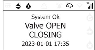
4 When the closing of the selected valve is completed, the LCD screen informs that it is **CLOSED**.
