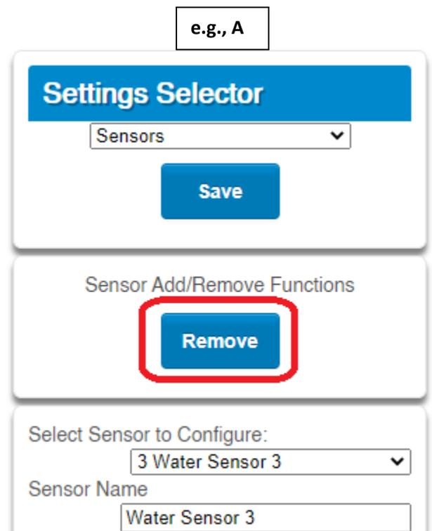
\*Before deleting a sensor, make sure that it is not in alarm, otherwise when you are going to reconfigure another sensor, your system will continue the alarm (Exception: **Lost sensor**)
